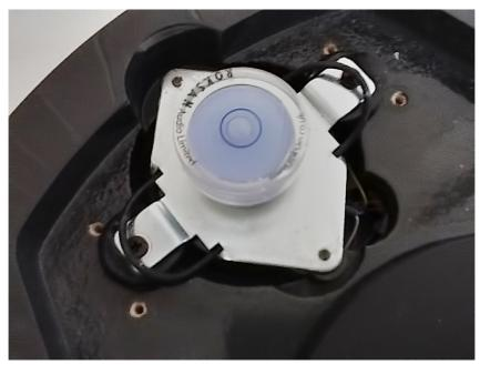
Using a spirit level to balance the motor mount (note the new grommets and black screws)
