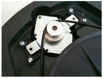
Motor mount - with platter removed
